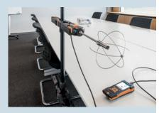
**Solution:** Integrated evaluation of climatic conditions with one multifunction instrument. Standard-compliant evaluation of the comfort level in accordance with PMV/PPD. Determination of the indoor air quality.
