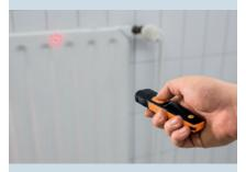
**Solution:** Non-contact temperature measurement.
