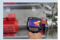
**Solution:** Early detection of wear via non-contact determination of the increase in temperatures in components.
