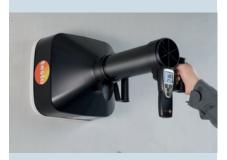
**Solution:** Precise flow measurement with a flow straightener.
