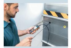
**Solution:** Measurement of flow velocity and volume flow in the ventilation duct.
