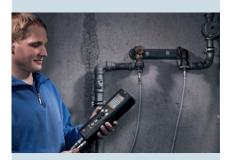
**Solution:** Tightness test using certified measuring instrument and digital documentation of the results as reliable evidence.
