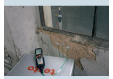
**Solution:** Simple measurement of the U-value provides information about the insulation characteristics.
