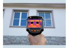
**Solution:** Thermographic visualization of the entire building shell using a thermal imager.
